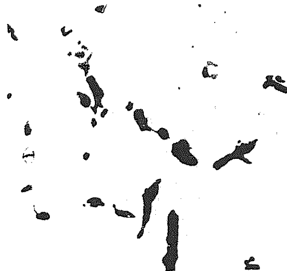
Fig. 13-9. Polished gray iron (Same as in Fig. 13-5 but not etched), showing the type of graphite flakes present in high-strength iron. Magnified 250 times.
