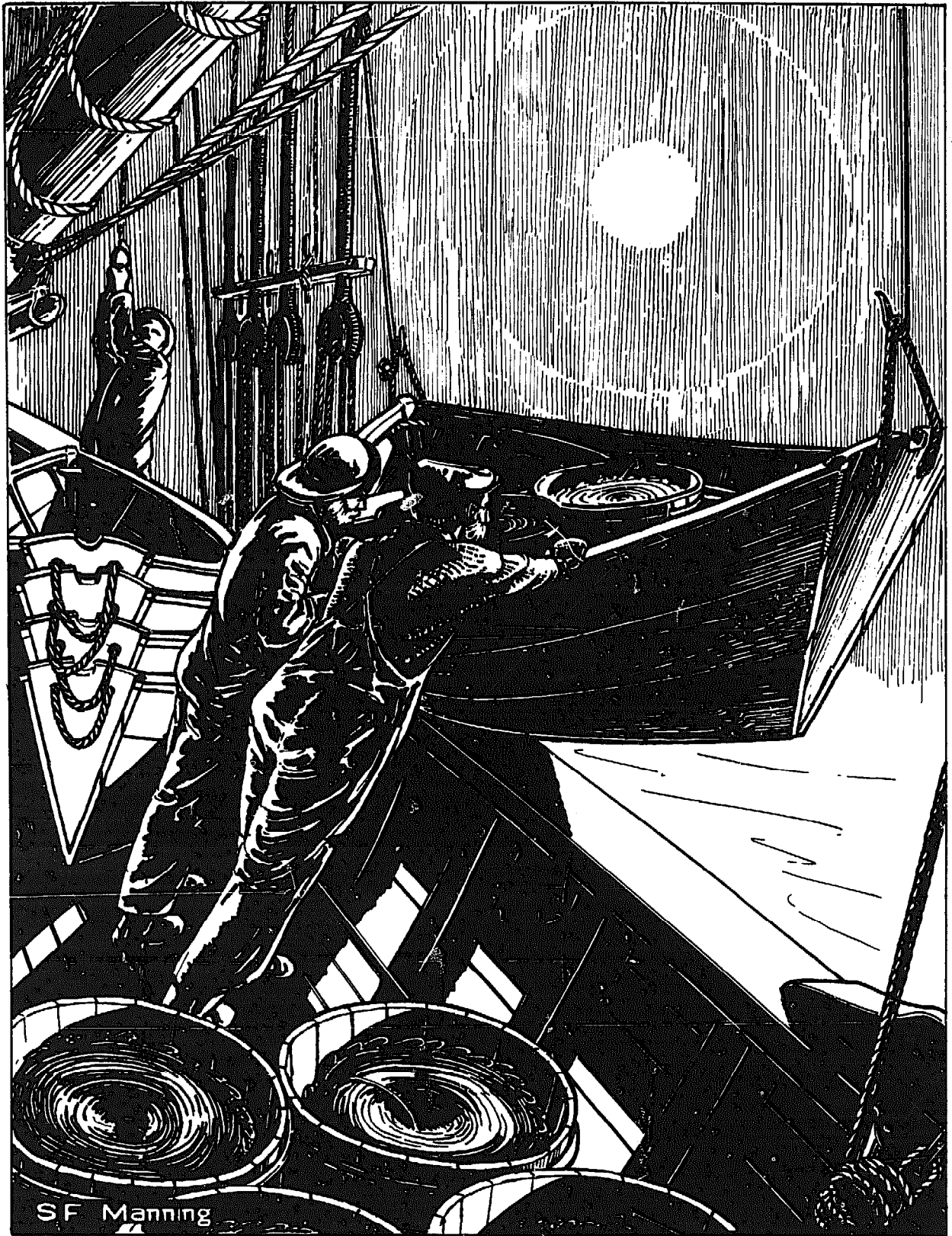
In a fishing schooner, the dories were hoisted in and out by tackles made up to the crosstrees of the schooner's masts. A hooked rod, or dory hook, at the end of the dory tackle permitted over-the-rail fishing for the rope buckets of a dory alongside.
