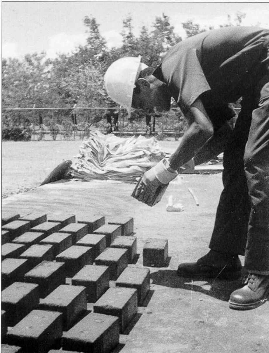
Fig. 1: Bricks produced with a CINVA ram and stacked on the ground for drying
