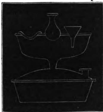
It will be seen that, from the steam-chamber being placed above the boiler, the condensed water is raised over and over again.
