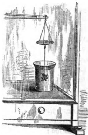
levelling the convex surface of the water at the mouth, to produce the same conditions as in the first weighing, it was placed in the balance-pan, and required 851.15 grains to equipoise it; but the weight of the bottle full of water without the gold being placed in it (814.20) plus the ascertained weight of the globules (38.95), amounts to 853.15 grains; and  $853.15 - 851.15 = 2.00$ , the weight of the water which overflowed, and
