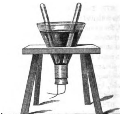
not to be used in eudiometrical researches, the boiling of the water may be omitted, and ordinary acidulated water be used instead. Of course the current must be allowed to pass until all the air is expelled, before collecting the gas.
