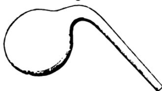
ture: when a sufficient quantity has entered, the point, *b*, may be closed by the blowpipe. This method is especially useful in experiments where it is wished to operate upon known quantities.
