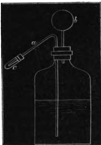
On applying pressure to the ball, the solution rushes up the tube *a*, and is forced into the burette or other vessel used to receive it. On removing the hand, the ball resumes its original shape, and a volume of air equal to the fluid expelled enters by *a*. The fact
