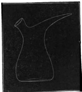
fitted with a good cork, may be used. The weight should be ascertained when empty, or, what is perhaps better, counterpoises for all the platinum crucibles, porcelain capsules, and other vessels in which weighings are to be effected, may be constructed from pieces of lead or brass; these being placed in the other pan of the balance, considerably facilitate the estimations.
