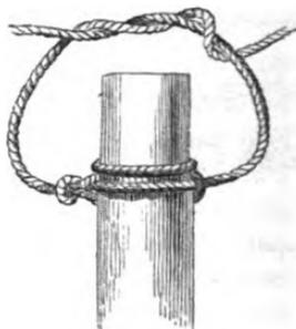
709. I have found the last of these knots useful in confining the stoppers of glass bottles in which reactions were to be effected by exposure to  $212^{\circ}$  in the water-bath, in cases where the use of pressure-tubes was objectionable from the small quantity of material which they were capable of containing without increasing their length to an inconvenient degree.
