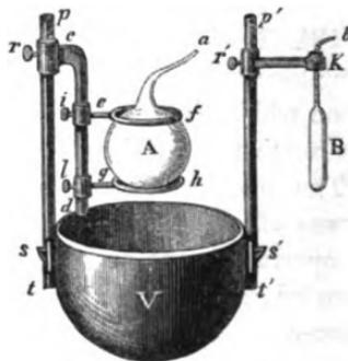
very necessary thing in many cases. The rod, *t'p'*, supports an arm, *r'K*, having a pierced cork at its extremity, serving to hold the air-thermometer, *B*, or a mercurial one, according as the temperature to which the bath is to be raised is more or less elevated.
