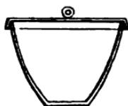
271. The capsule, fig. 149, is also adapted for ignitions and fusions, but is more appropriate to evaporations and crystallizations on the small scale, especially those in organic research.
