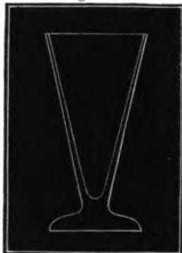
a considerable size. They are sometimes made of the same shape as that represented in fig. 103, but blown at the lamp and exceedingly thin, and thus resemble a test-tube on a foot; they are very convenient in many experiments of a delicate character.
