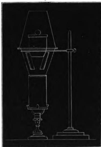
and others, that it is seldom necessary to use Sefström's blast-furnace. Where the full powers of a lamp are required to be exerted, the crucible jacket, fig. 33, is necessary; it will be seen that the crucible is supported on three knife-edges; the arrangement is such that the flame is made to act on the crucible in a manner well adapted to economize the heat and avoid loss by radiation.
