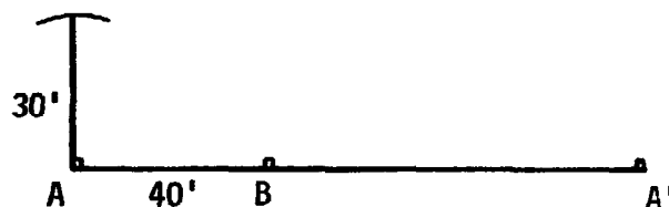
FIGURE IX-A. LAYING OUT A RIGHT ANGLE
