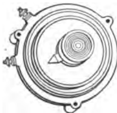
FIG. 150. — View of field rheostat with its connections.
