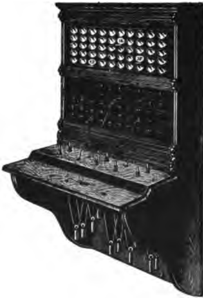
FIG. 385. — Simple form of switchboard for small exchanges.
