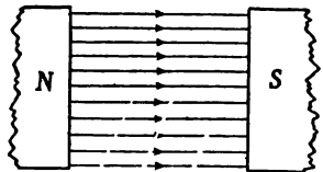
FIG. 163. — Uniform magnetic field.
