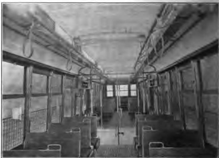
FIG. 358. — Large semi-convertible prepayment car with powerful motors. The center entrance makes this car also convenient to use as a trailer.
