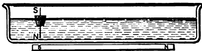
FIG. 41. — Experiment to illustrate the movement of a free magnet pole when near a bar magnet.
