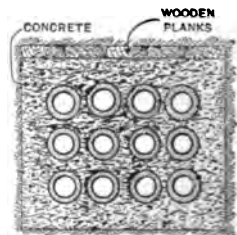
FIG. 301. — End view of conduit containing twelve ducts.
