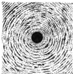
FIG. 44. — Iron filings showing the distribution of magnetism around a wire carrying an electric current. The black dot represents a cross section of the wire.
