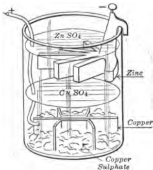
FIG. 11. — Gravity or crowfoot cell.
