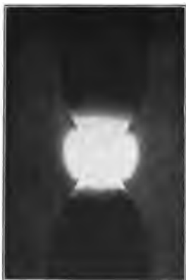
FIG. 321. — Open arc produced by alternating current.
