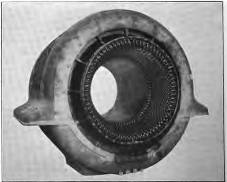
FIG. 237. — Stationary armature of figure 236 for high-speed alternator.
