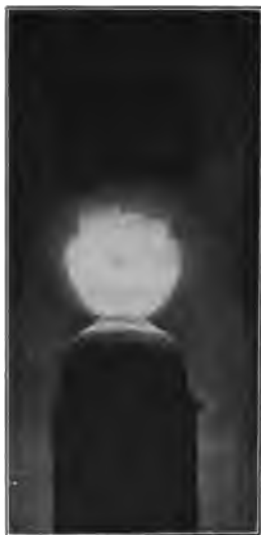
FIG. 320. — Electric arc produced by direct current.
