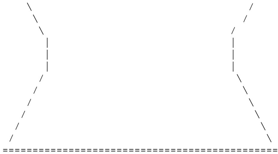
In particular, this sounds like a pincushion problem - to correct for pincushion, a signal from the vertical deflection that looks something like a rectified sinewave is used to modify width based on vertical position. There is usually a control to adjust the magnitude of this signal and also often, its phase. It would seem that this circuit has ceased to function.
