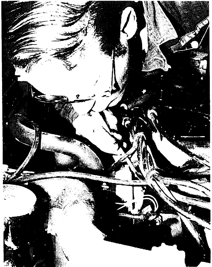
If you don't have compressed air for blowing dirt out of the spark plug ports, use a straw and your lungs.
