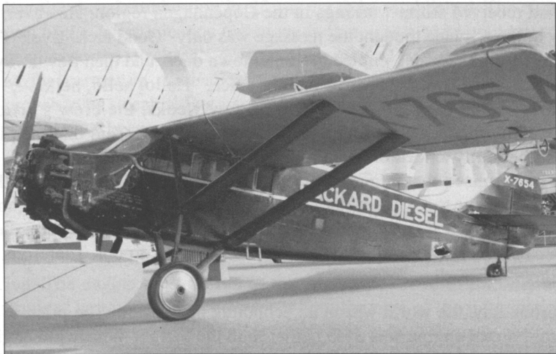
Photo 33-3 Stinson plane mounting Packard diesel engine: The Stinson plane was painted black to make the soot staining due to exhaust gas from the Packard engine inconspicuous (Ford Museum).
