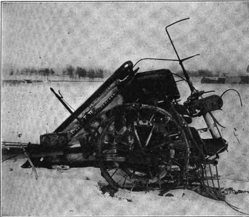
FIG. 223.—A corn harvester left out in the snow to rust and decay. This is a great loss to the farmer and should be avoided.
