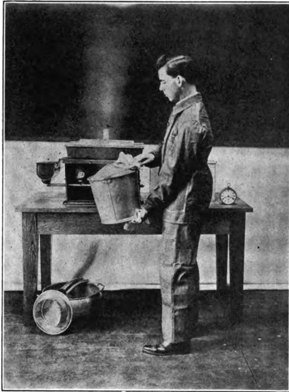
FIG. 171.—Simple and inexpensive steam sterilizer, consisting of a roasting pan with a special cover which can be made by any tinsmith.
