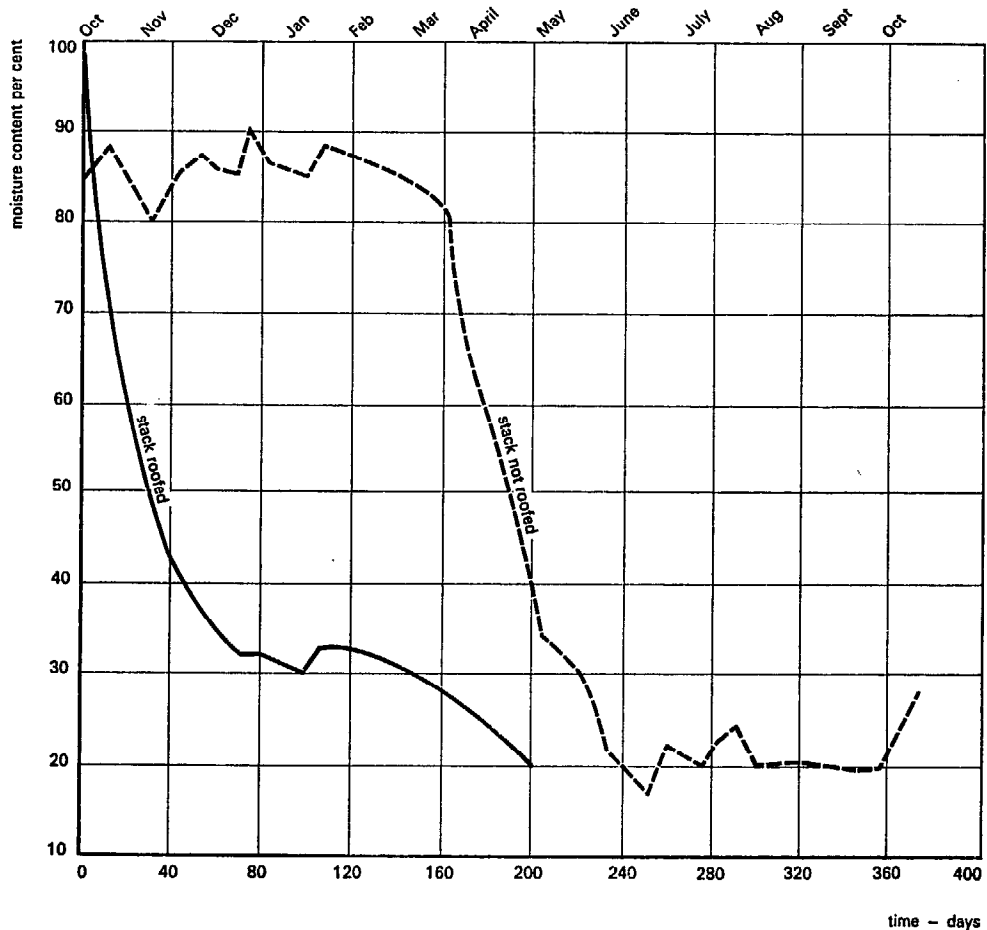
Figure 8 Effect of roofing on rate of drying 100 x 50 mm Sitka spruce in W. Scotland
