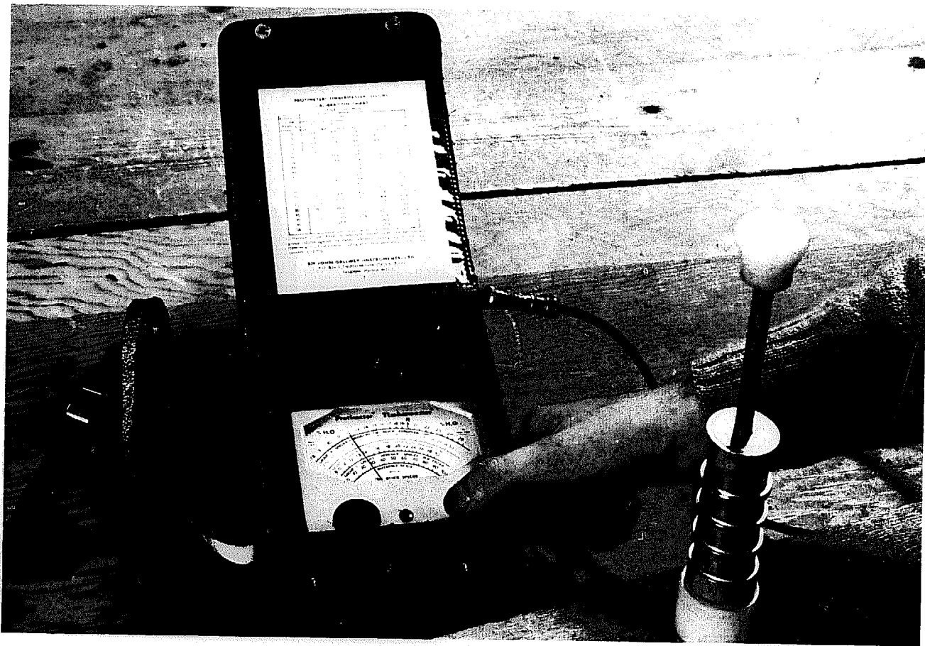
Plate 3 Moisture meter and hammer-type electrodes
