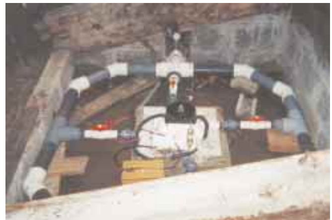
Llano's ES&D 28 volt DC alternator acted as the control group in the comparison of AC induction generators.
