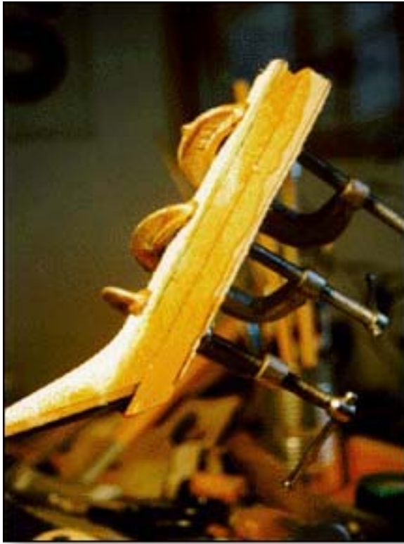
Spruce ears being clamped on. Finished ears after shaping.
