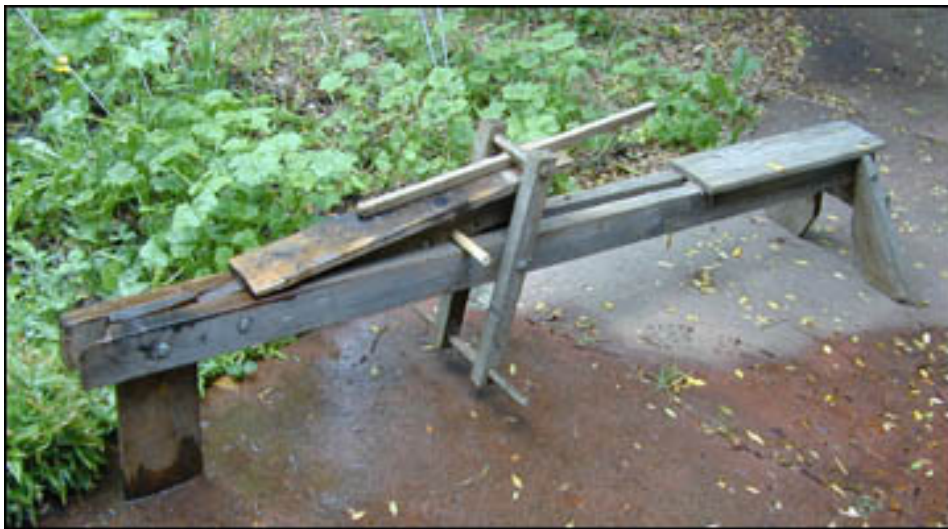
Foldable shaving horse made of 2 x 4's and scrap wood.
