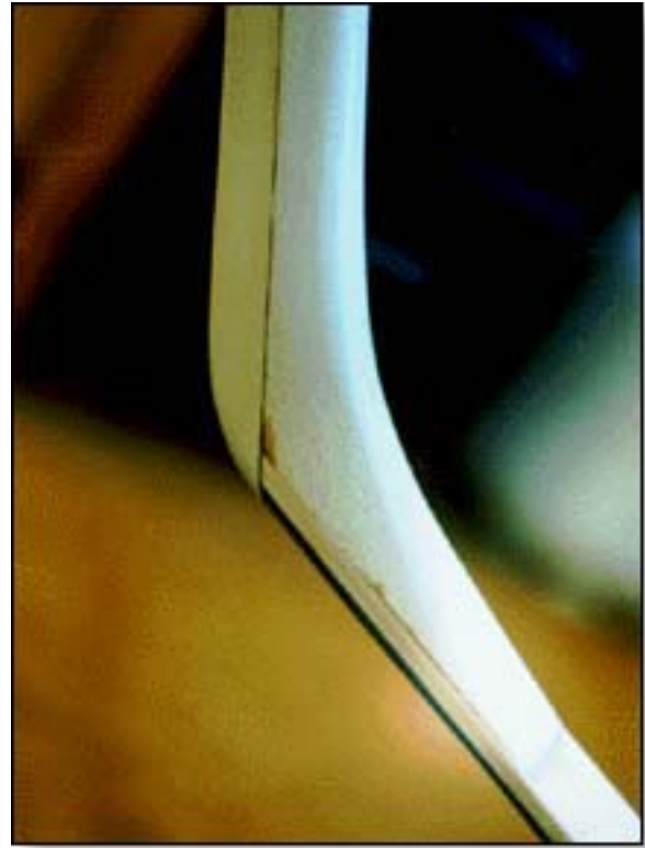
Spruce ears being clamped on. Finished ears after shaping.
