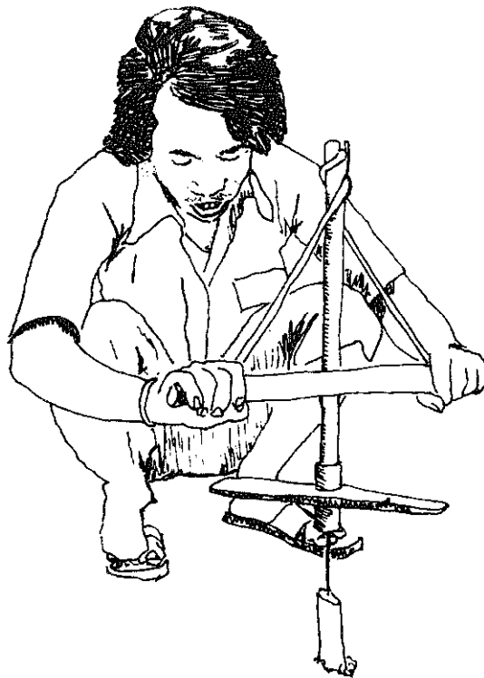
Drilling a buffalo horn knife handle.
