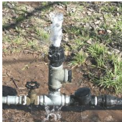
A basic version of the "Hi-Ram Pump" (The steel pipe on the left is the drive pipe entering the pump)
