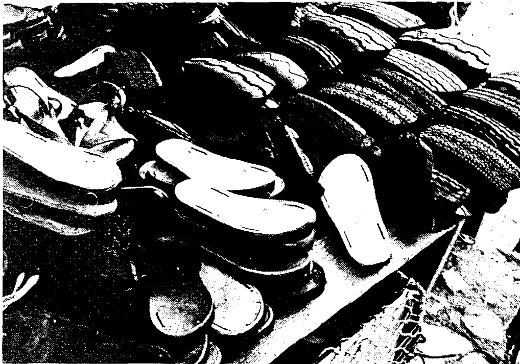
Fig. 59a Tyre tread is used for sole grip. Note the leather insole and slots for sandal straps. Such sandals will last five or ten times as long as a mass produced plastic one. Photo: courtesy of Oxfam.
