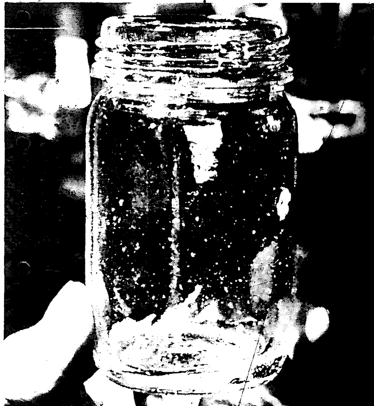
Fig. 62 This jar is very 'seedy' due to the use of nearly 100% cullet in its manufacture.
