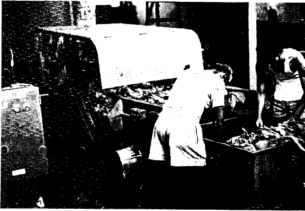
Fig. 55b The rag pulling machine is fed by loading rags on to the conveyor behind the man in the centre. Note that all moving parts are covered by guards. India.
