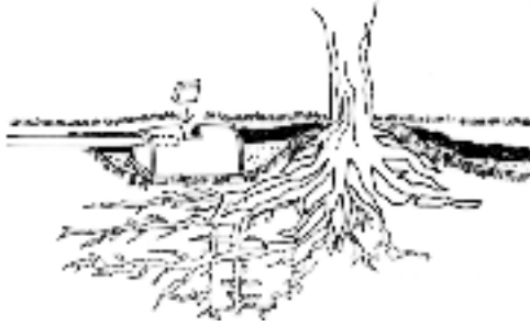
Figure 6.4 An example of direct use. The water is piped to a bed where it is applied below a mulch surface and is available for plants or trees. 7
