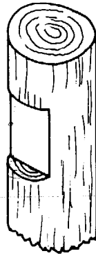
FIGURE 53 ROUND POLE NOTCHED FOR SAWN FRAMING MEMBER.
