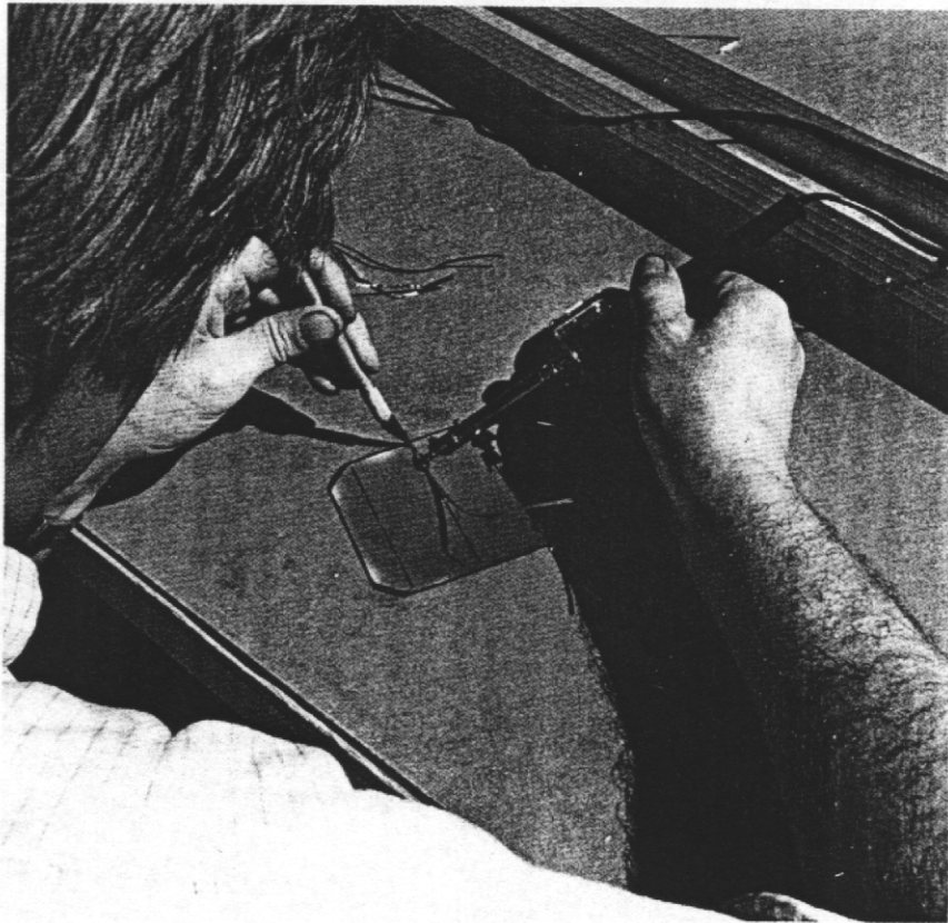
FIGURE 4.4—Soldering copper strips to a solar cell (David Ross Stevens photo).
